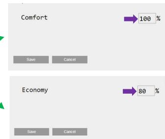
Due to the chosen method of air volume control, we distinguish two menus. The first one is for setting for fixed fan speed and the second one is for setting of the constant pressure control or for setting of constant flow control.
